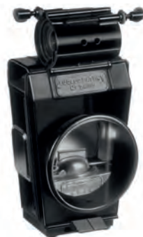
Circa 1882 Joseph Lucas & Son 'King of the Road' hub lamp as used with an Ordinary Bicycle
